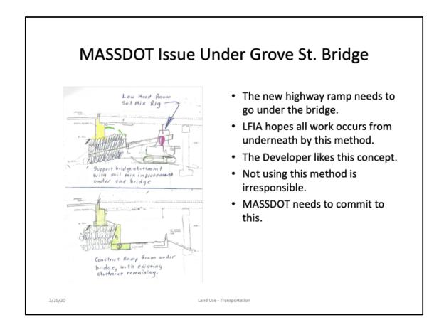
We favor: New access ramp from 128 northbound that passes under the Grove Street bridge in the sloped section under the existing yellow abutment.
