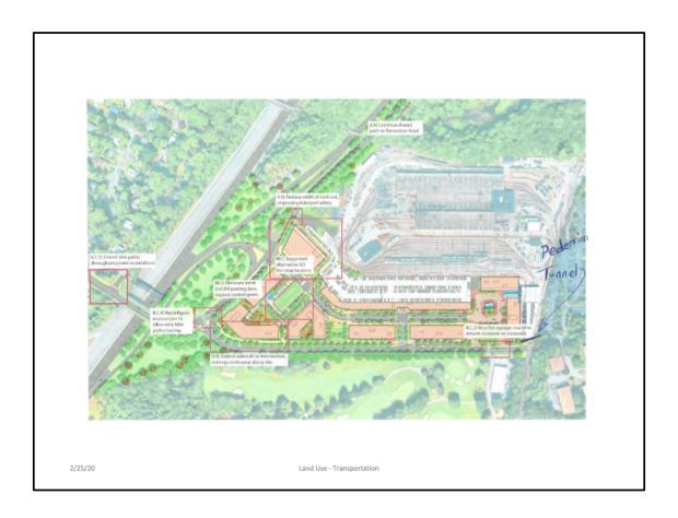
This slide shows an opportunity to connect possibly a pedestrian way through a small tunnel under the tracks, at the site grade, as required of the Riverside office Center owner, per their special permit, but only if Riverside is developed.
